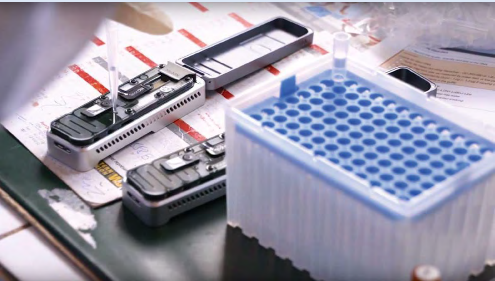
A handheld DNA sequencer being used in Madagascar to identify TB resistance in sputum samples Institut Pasteur de Madagascar
